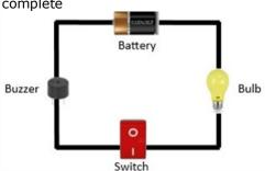
This circuit is complete so the buzzer will sound and the bulb will light.
